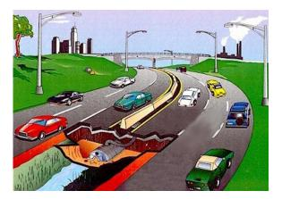
Onsite percolation controls capture stormwater from streets and percolate it into the ground
