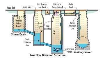
Low flow diversion structures capture dry weather urban runoff in the storm drains and pump it to the wastewater collection system
